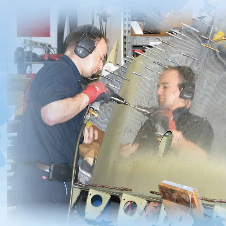
Ben and Chuck (hiding below) team-rivet a shiny new skin onto the 182 wing.
