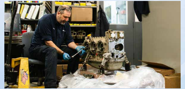
Josh disassembles an engine that has arrived for overhaul.
