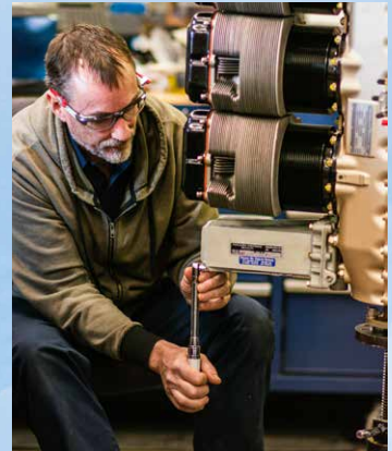
Josh disassembles an engine that has arrived for overhaul.
