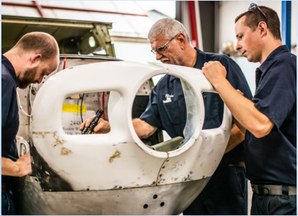
Chris, Phil, and Ben perform a dye penetrant inspection on the 206's engine mount.
