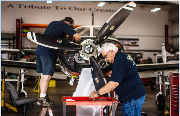
Jay and Gary (a volunteer) wrap up the engine inspection on the Piper Malibu.
