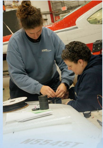
Rebekah, one of our avionics specialists, teaches Brittany how to neatly bundle wires for installation in the airplane.
