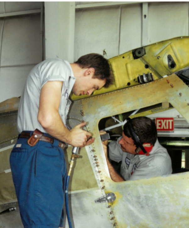
Above: Chris Jutte guides apprentices Phil Sperling and Ben Plitt Bottom Left: Chuck Egbert and Chris Jutte team rivet as apprentices in the late 90s. Both are now MMS staff. Right: Chris Jutte makes repairs to a wing
